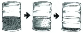
3. Reuse water wherever possible (i.e. back into a batch or mix process). Otherwise, as last resort. adjust pH to neutral and dispose of as trade waste water. (Disposal of any type of wastewater to sewers must first be approved by the local Water Authority). Excess concrete slurry should be allowed to set and taken to a recycling yard with other recyclable materials from a building/construction site.
